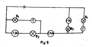
In the above circuit, *B1*, *B2*, *B3* and *B4* are bulbs. The readings of ammeters E and F are respectively
