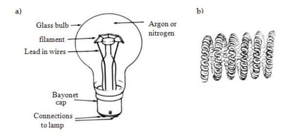
Most lamps are gas filled and containing nitrogen or argon not air. This reduces evaporation of the tungsten which would otherwise condense on the bulb and blacken it.
